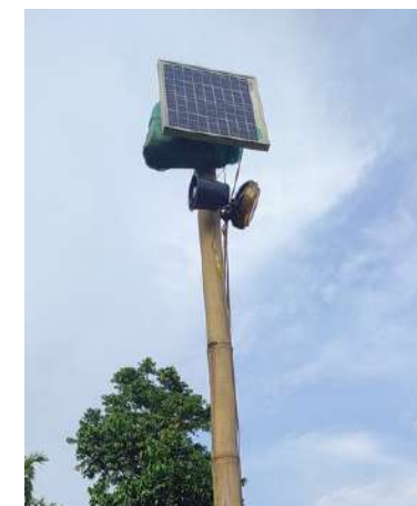
'Alarm fence', an early warning system to warn people of elephant entry into tea-plantation housing.
